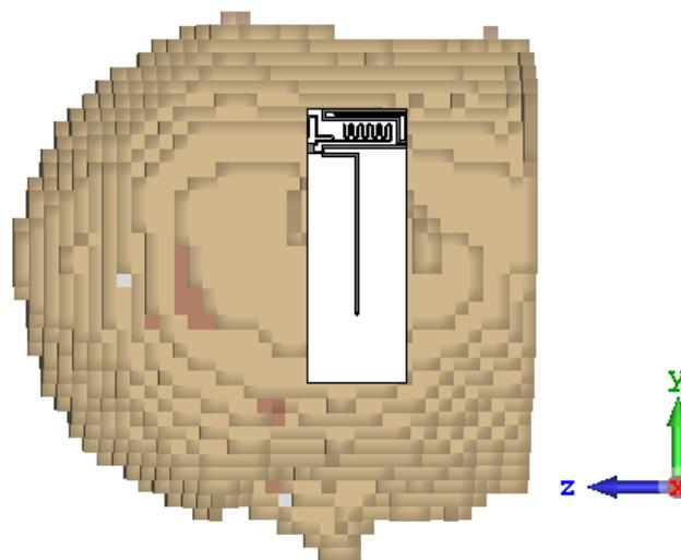
Fig. 6 Antenna structure with the human head model (Hugo voxel model)
