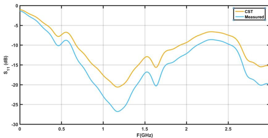
Fig. 3 Simulated and measured return loss of the proposed antenna.
