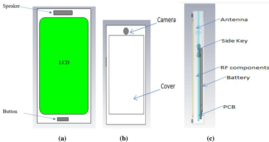
Fig. 4. Structure of mobile (a) Front, (b) Back, and (c) Side view
