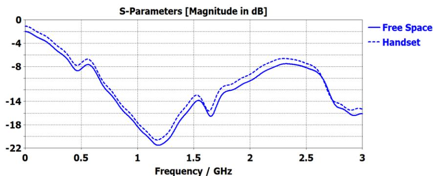
Fig. 5 Comparison of return loss of antenna in free space and handset
